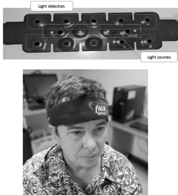
Figure 3. In the top picture, the fNIRS sensor pad includes light sources (in orange) and detectors (in red). Infrared light is absorbed by hemoglobin in the blood stream. Oxygenation is calculated from the difference between emitted and detected light. The bottom picture shows a participant with the sensor pad placed on the forehead, where it will capture oxygenation of the prefrontal cortex.
